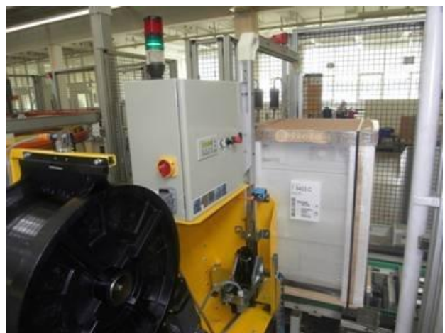
MH-V model in operation at the end of a packaging line securing packed appliance products
