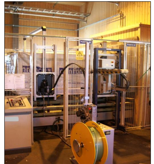
Lumber Hood strapping with 9-12 mm PET strap to secure the load cover
